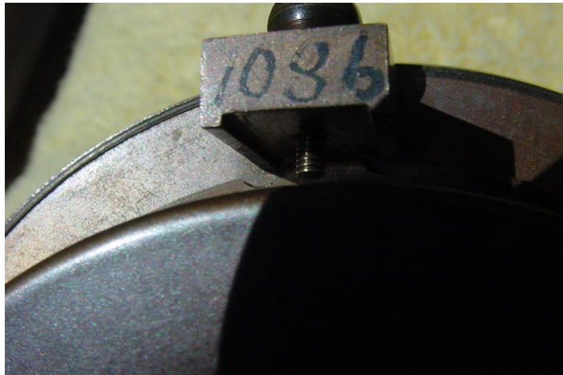
Photo 11, showing serial number marked on movement mounting block. Some clocks have the markings on top of the mounting post as well.
