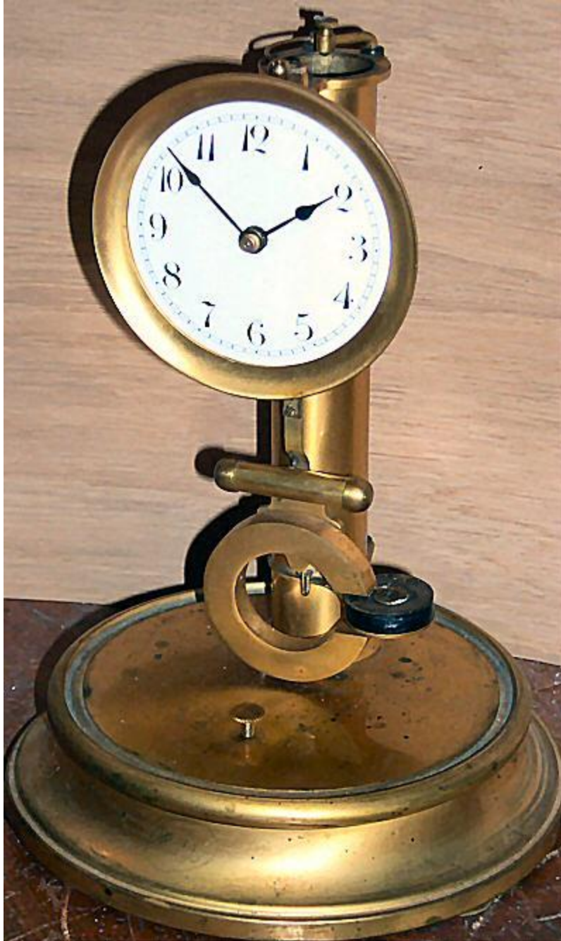
Photo 9, Henry Warren production Mystery clock S/N “4051” (there is doubt about the authenticity of this serial number since it is written in pencil and not in the usual places) with a magnetically coupled pendulum driving synchronous, oil-filled “motor” with sealed drive gears.
