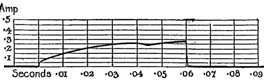
Observe the clean "make," and precipitous "break." When the current has risen to .25 amp.—and it takes 4/100ths of a second to reach it—all the dials operate, and the little dent or depression shows they have done so. Not until the current has risen to a higher figure is the switch automatically thrown open. Thus the switch is bound to transmit sufficient electrical energy to operate every dial; it cannot work at all without doing so.
