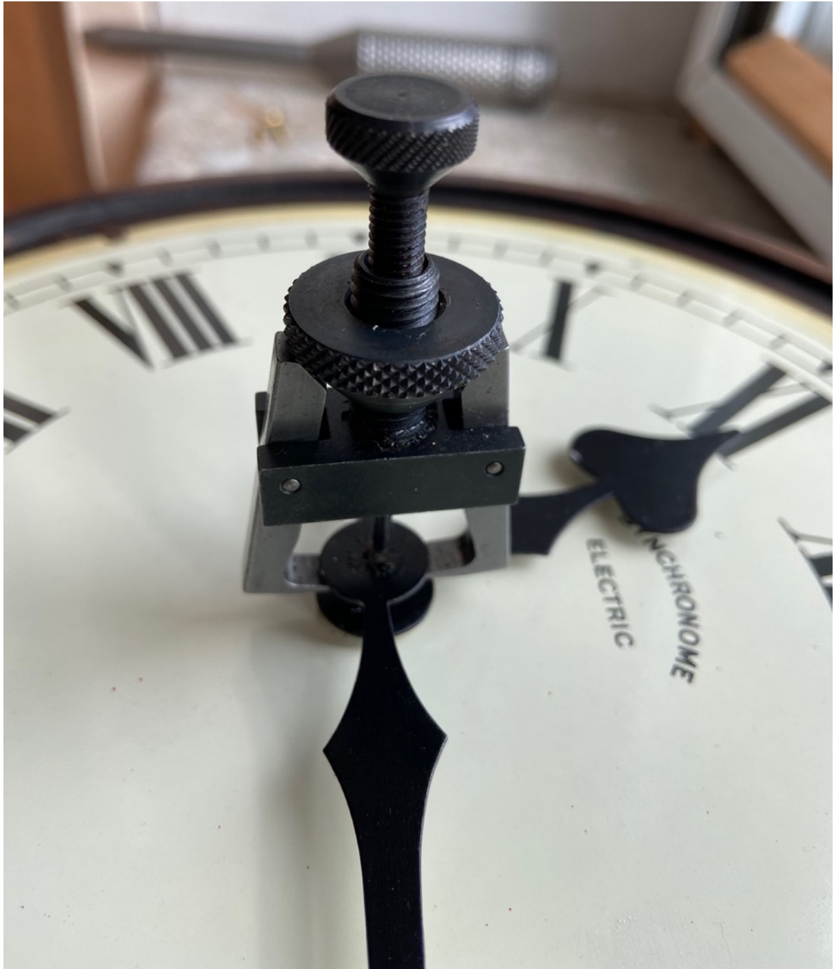
Figure 3 – Using a hand puller to remove the minute hand.
