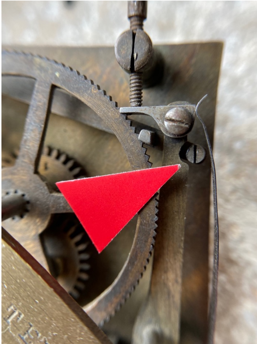
Figure 10 - Double locking movement – detail showing additional locking.
