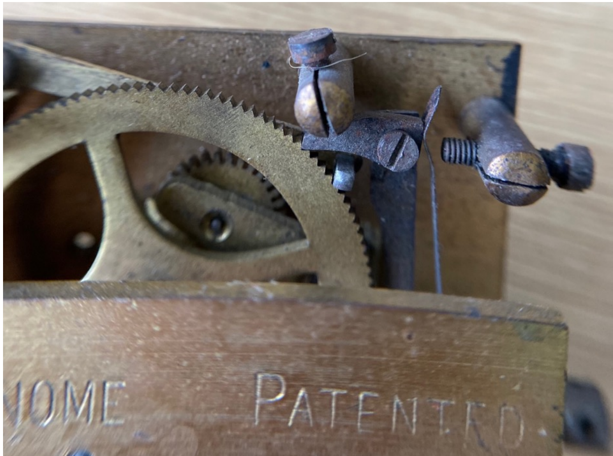
Figure 11 - Small (No 1) movement showing adjustments.
