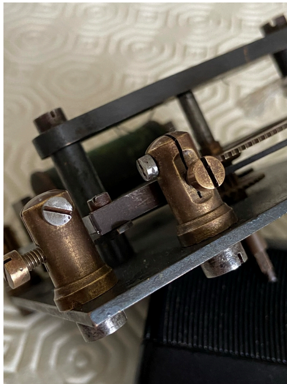
Figure 4 - Detail showing thickness of bridge and back plate
