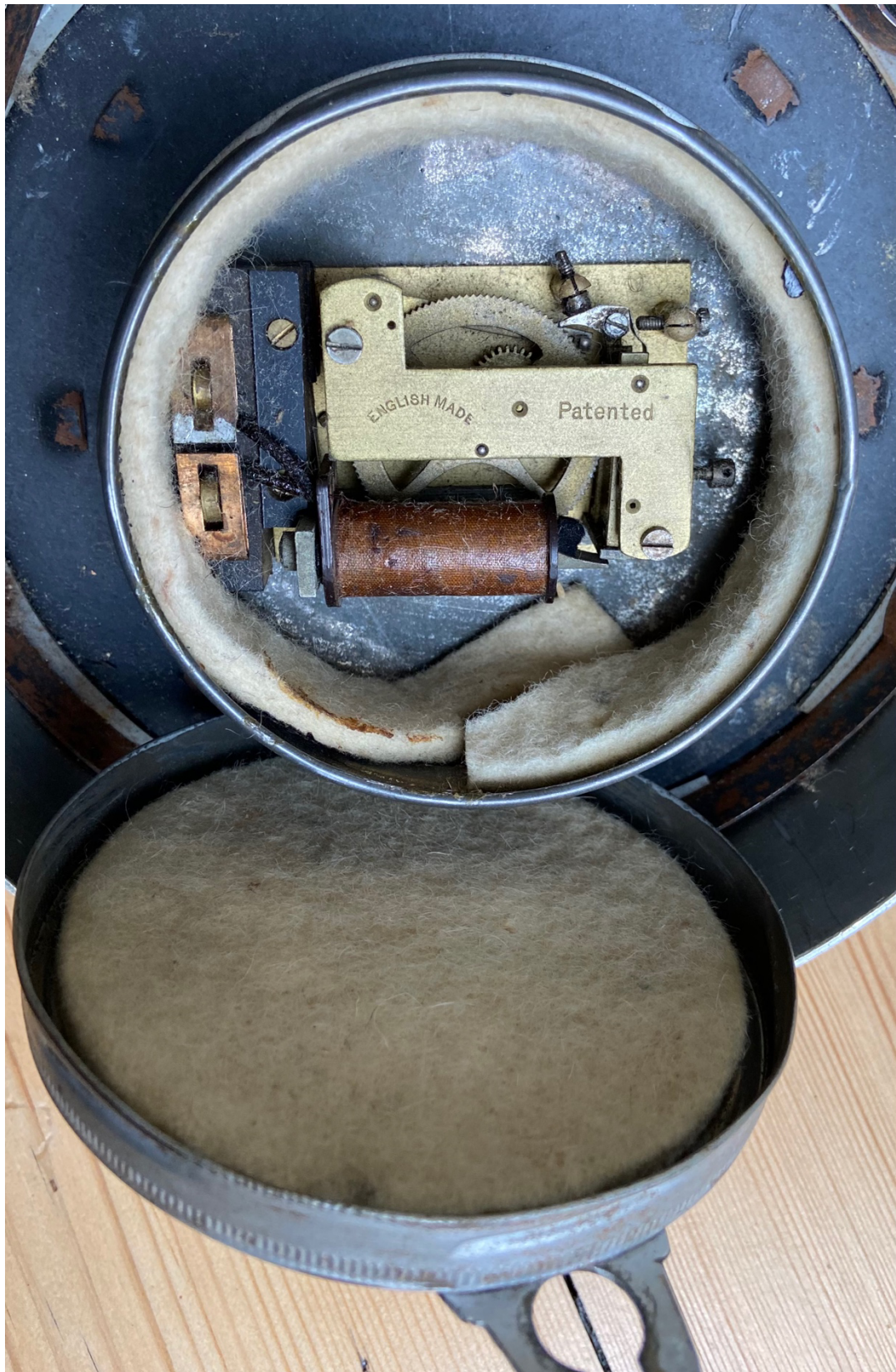
Figure 20 - Silent movement in insulated can.
