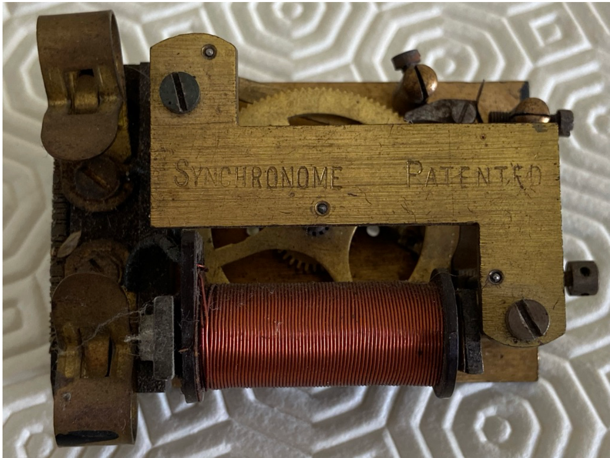
Figure 16 – Standard (i.e. 'normal' armature) No 1 movement
