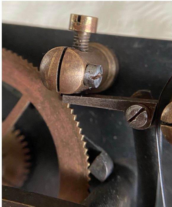
Figure 3 - Detail of adjustment lock screws
