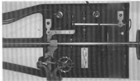
A typical Brisbane-made controlling pendulum (C.P.) A cast iron frame carries the mechanism and is extended up to support the pendulum suspension. The mounting of the impulse pallet on the
