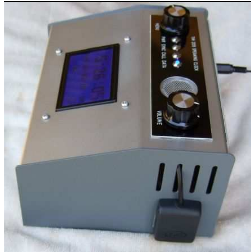
GPS receiver module fixed outside the casing
