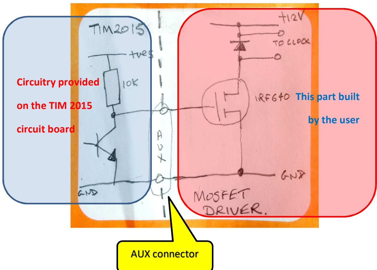
The MOSFET is an **IRF640**. The recommended diode is either a **1N4004** or **1N9004**.
