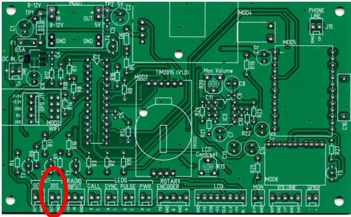
You can fix a pair of wires fitted with a Molex or Dupont plug on the pins of J4 and connect them to two pins of the auxiliary (AUX) connector on the back panel of the case. All pins on the AUX connector are ‘user-assignable’, so you are free to choose any two pins as you please.
