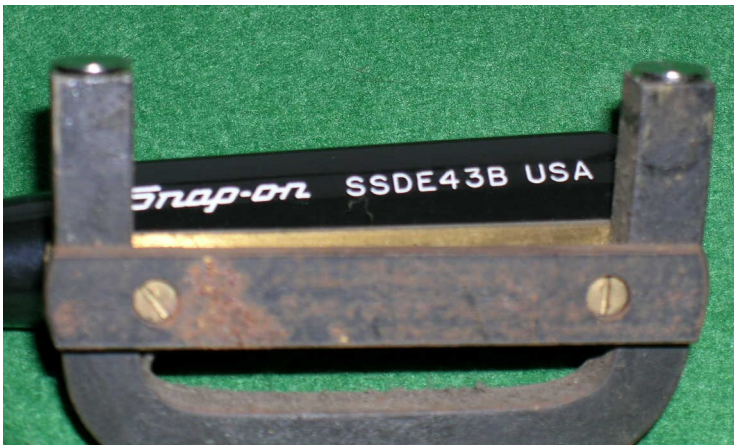
Figure 8 - New magnets in place on old magnet
