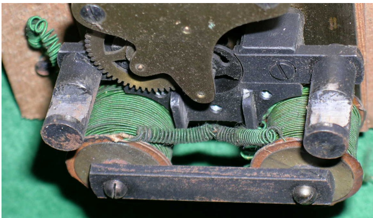
Figure 4 - pole piece receptacles on the stator assembly
