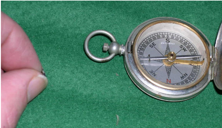
Figure 7 - Checking the polarity of the new magnet
