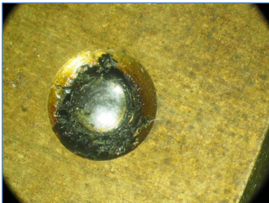
Figure 28: Count wheel rear pivot 'as found'
