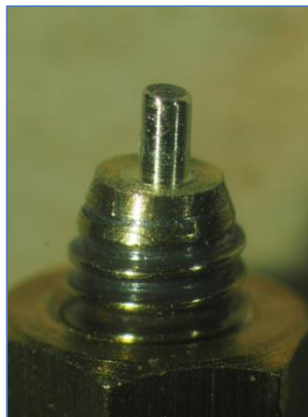
Figure 46: Solder turned off to reveal spigot
