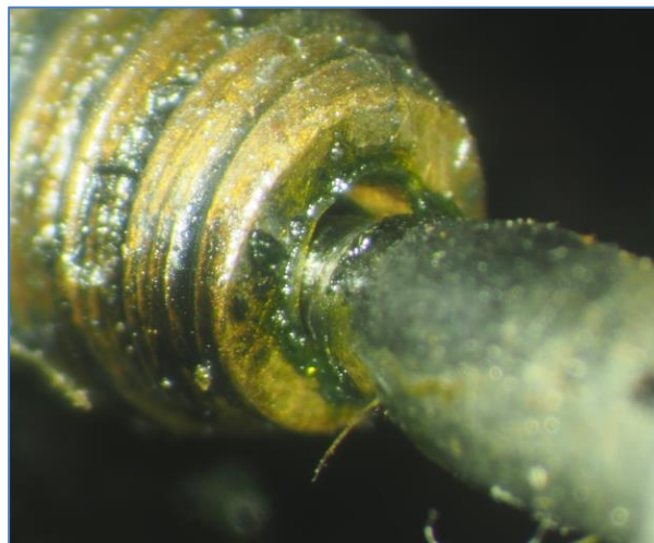
Figure 27: Hipp-toggle rear pivot and bearing as found
