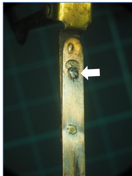
Figure 35: Soldered contact removed to reveal a steel contact (arrowed)
