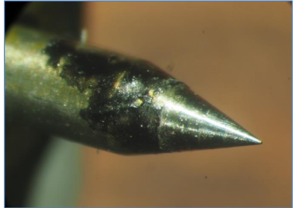
Figure 26: Advance pawl rear pivot showing paint deposit
