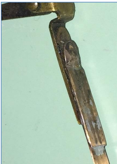
Figure 34: Dial contact before treatment, with added contact spring
