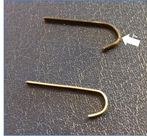
Figure 68: Broken spring (top) and new replacement part (below)
