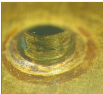
Figure 20: Wear to front crutch pivot hole
