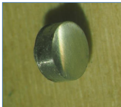
Figure 39: New domed and polished platinum contact
