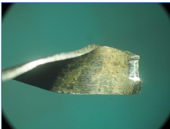
Figure 30: Wear to working surface of click
