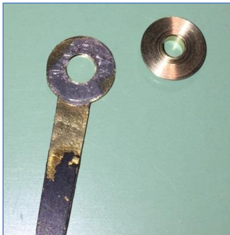
Figure 54: Minute hand with new collet
