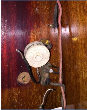
Figure 63: Dial spark quench resistor 'as found'
