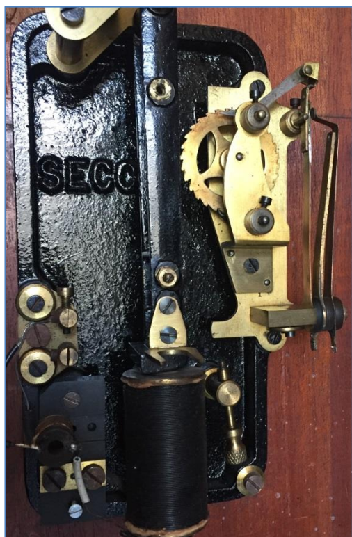
Figure 16: Movement 'as found' with gloss paint (pendulum not fitted)
