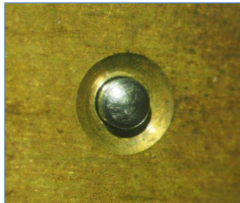
Figure 29: Count wheel rear pivot after treatment
