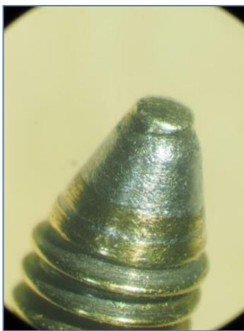
Figure 45: Lower contact screw with brass spigot protruding through soft solder
