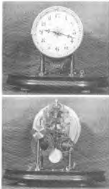
Dome covered striking mantle model. Upper, front view with dome removed. Lower, back view showing movement.
