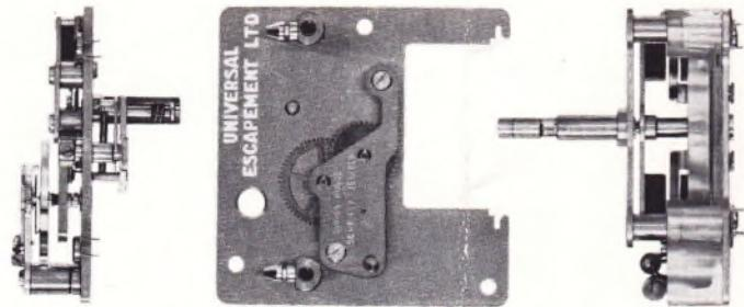
The Escap system consists of two units easily interchangeable: the escapement and the motor, both mounted on the holding plate.
