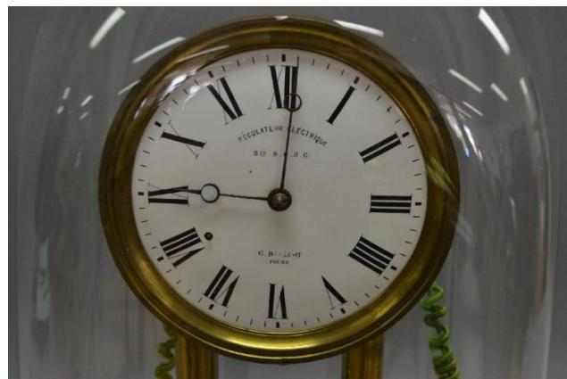
Nor was the condition of the clock indicated in the description and only by visual examination could the problems be determined. With on-line research prior to the auction I was able to establish that the entire electric solenoid and the remontoire lever system were completely missing. The Clockdoc website (<http://wp.clockdoc.org/>) contained pictures of similar clocks by Reclus and from those I was informed enough to make a winning bid for the clock.
