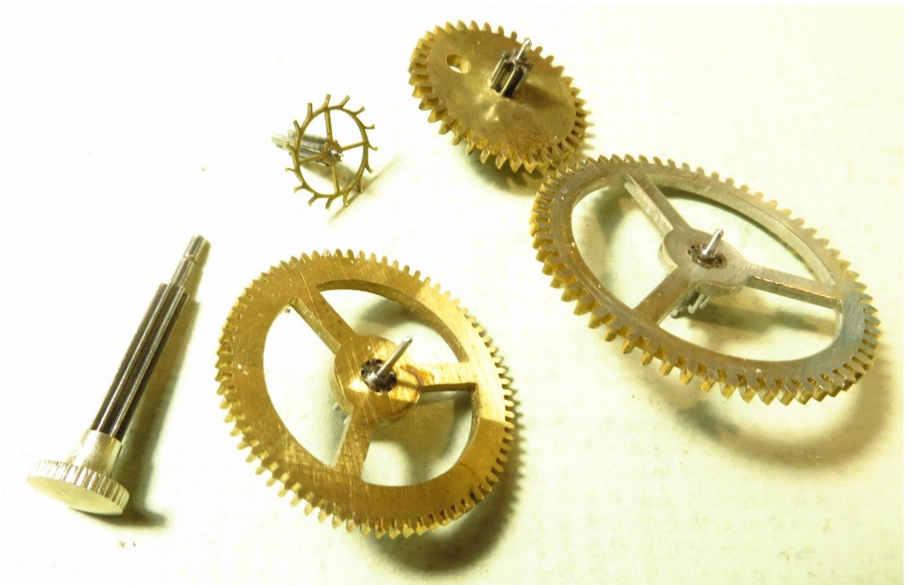
Most rust was relatively superficial and with light pivot polishing bearing surfaces were rendered smooth.
