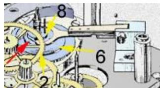
*angled ring* at the base of the driver and release nut (red arrow) carries the forked extension of one of the switch arms. As the barrel drives the movement, it rotates clockwise (as seen from the top plate, as illustrated), gradually raising the forked arm (onto the higher
