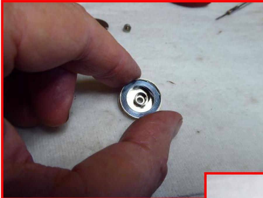
25. With the spring in the barrel, refit the arbor and close up with the barrel cap.
