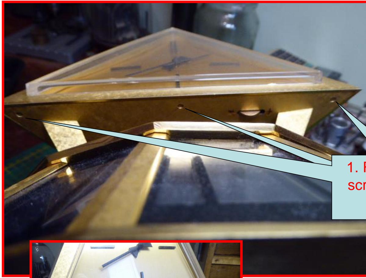
1. Remove these 6 screws from under the pyramid
