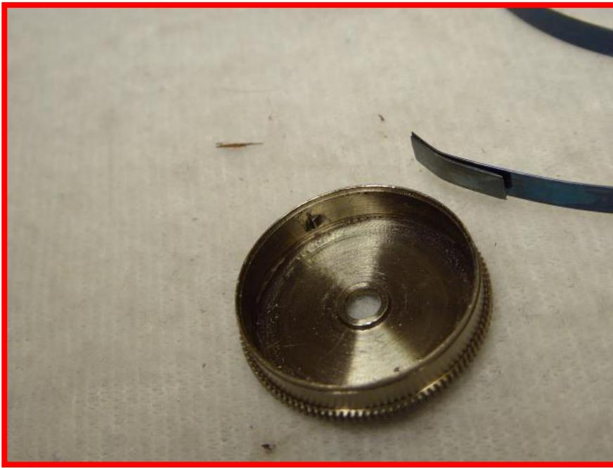
Note: the hook end of the spring locks behind a small hook on the barrel wall.
