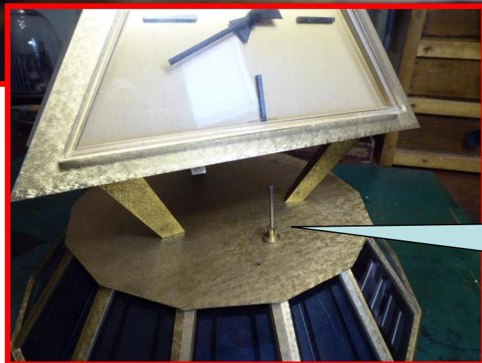
You will need a very short screwdriver to fit the centre screws under the pyramid.
