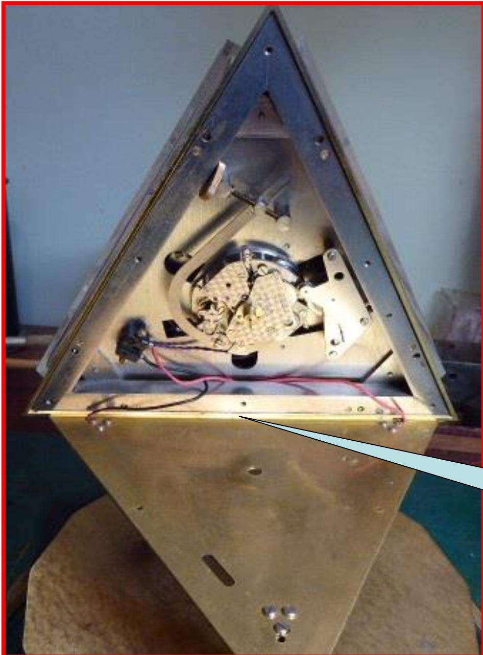
With the 6 screws removed the pyramid may be tipped up.
