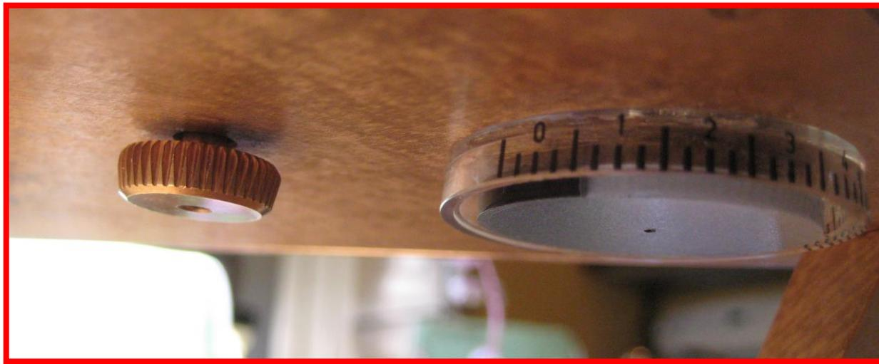
The problem here is that the indicator disc will not be fitted until the entire pyramid is assembled. To overcome this I determined the position of the pin such that it had 7 days to reach the micro-switch.
