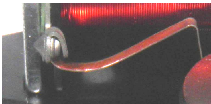
FIGURE 1.2: Magnified view of fusible links in Kienzle type 607 clock. Fusible link at left appears to have partially failed already. Right-hand picture shows an intact fuse assembly.
