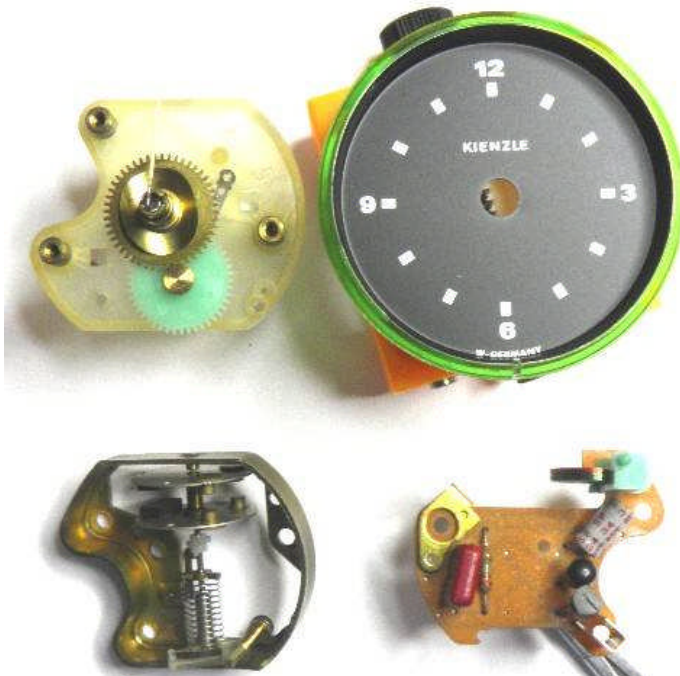
FIGURE 2.3: Major sub-assemblies of a Kienzle impulse clock. Clockwise from upper left:
