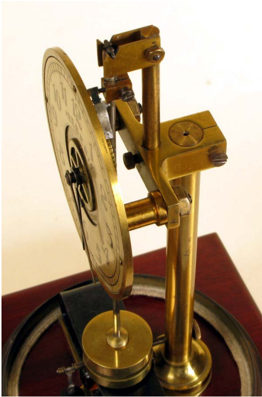
Fig. 12. Frame machined from solid.
