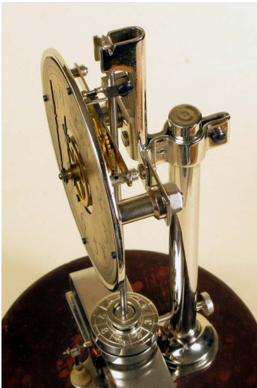
Fig. 13. Construction using pressed brass.
