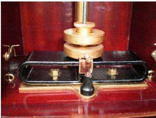
Fig. 9. Close-up of the coil, magnets and contact arrangement.
