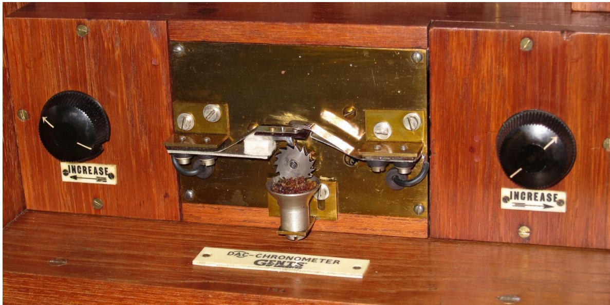
Fig. 20 Lubrication cup/bucket required to lubricate the teeth of the contact wheel
