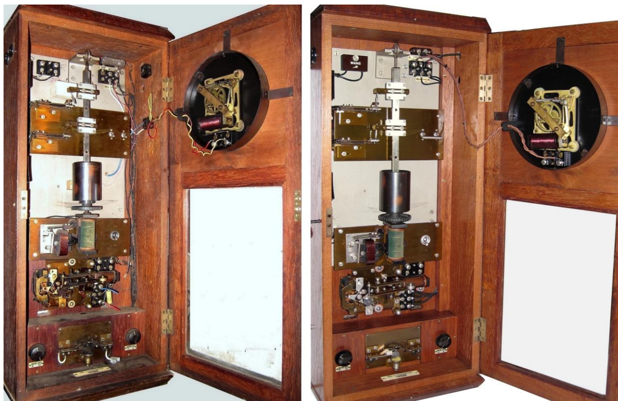
Fig. 27 DAC Chronometer with pendulum back-up, before restoration and after.
