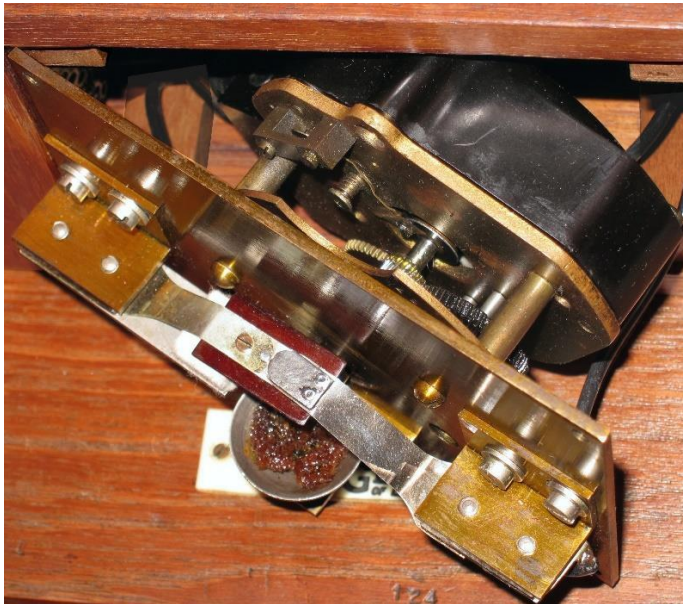
Fig. 18 Smiths synchronous motor, note lubrication cup/bucket
