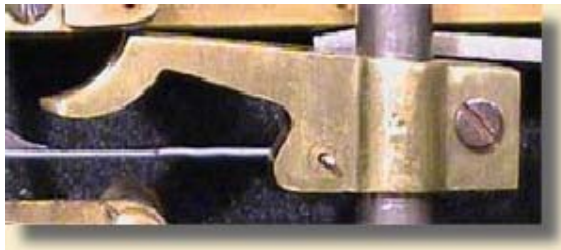
Figure 12 - Impulse pallet up to end of 10,000 series
