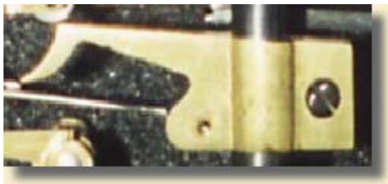
Figure 14 - Impulse pallet 10092 - example of a steeper slope
