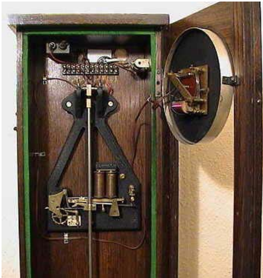
Figure 26 - ECS master - movement
