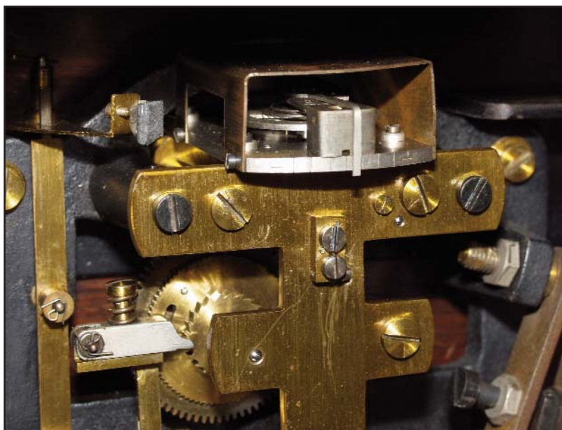
Figure 32. A close-up of the balance wheel escapement of the Pulsynetic movement shown in Figure 31.
