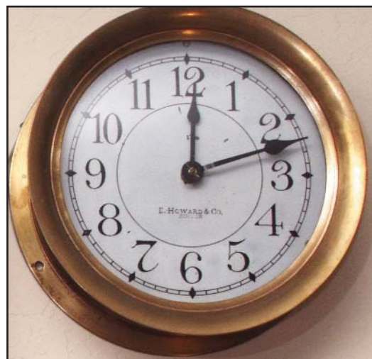
Figure 37. A Howard 10" brass case slave clock for marine application.
