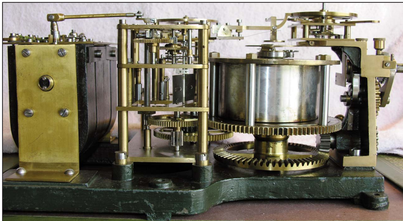
Figure 7. Side view of a Magneta movement showing horseshoe magnets (with coil inside) on left, mainspring on right, and clockwork with remontoir in middle.
