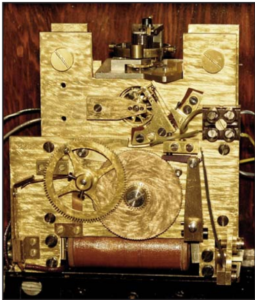
Figure 22, left. Typical Mercer electrically wound 30-second impulse movement with a horizontal platform chronometer escapement.
