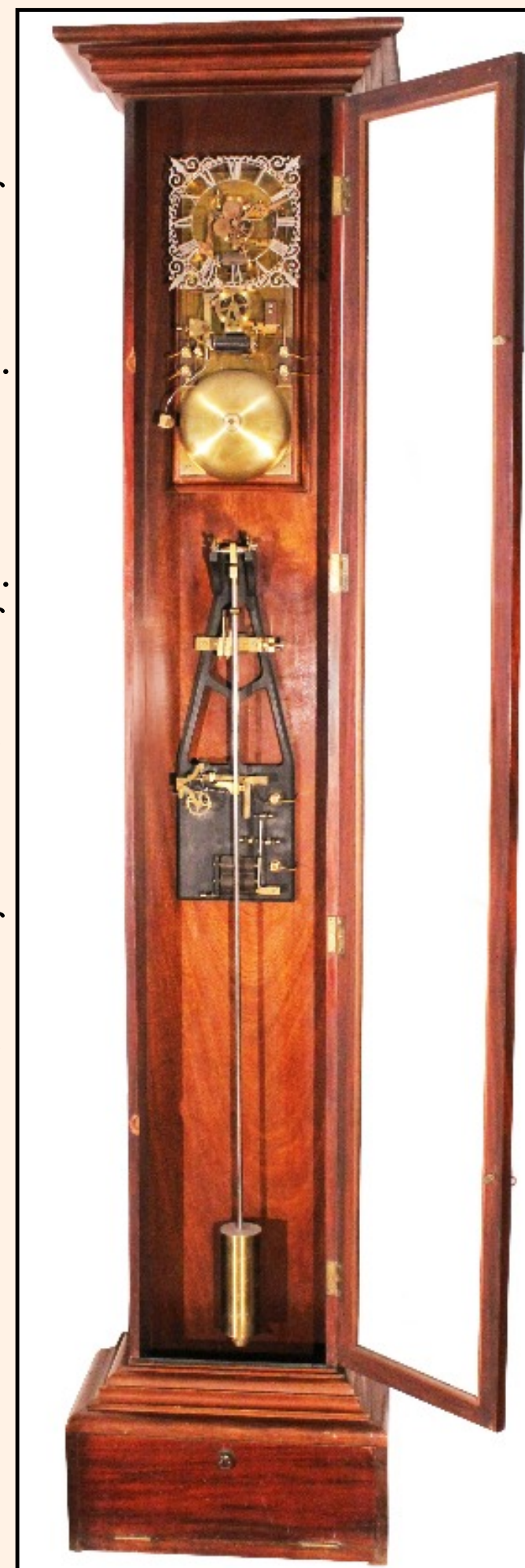
You can see the dial is completely skeletonized with matching filigreed hands, The hands are counterbalanced.
