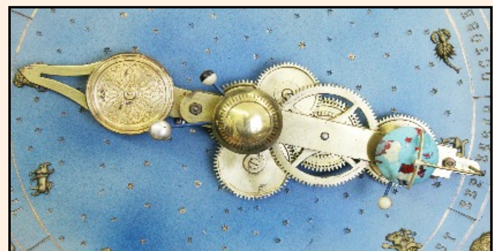
Left and Right: Illustrating the movement of the planets around the sun, the rotating Earth and movement of the Moon around the Earth as the entire orrery assembly rotates around the dial.
