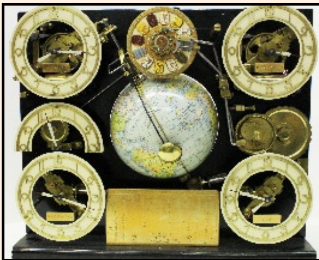
These pictures (above and below) show the movement of the Sun illustrating the Earth's declination. You can see the Equation of Time dial also move in conjunction with the Sun's movement
