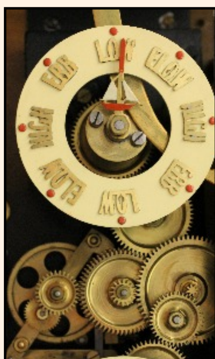
(Below) The Tides dial and associated gearing. The hand is in the shape of a sailboat
