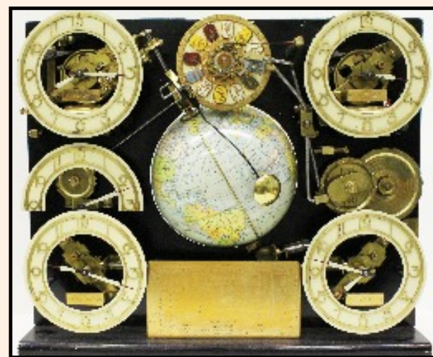
These pictures (above and below) show the movement of the Sun illustrating the Earth's declination. You can see the Equation of Time dial also move in conjunction with the Sun's movement
