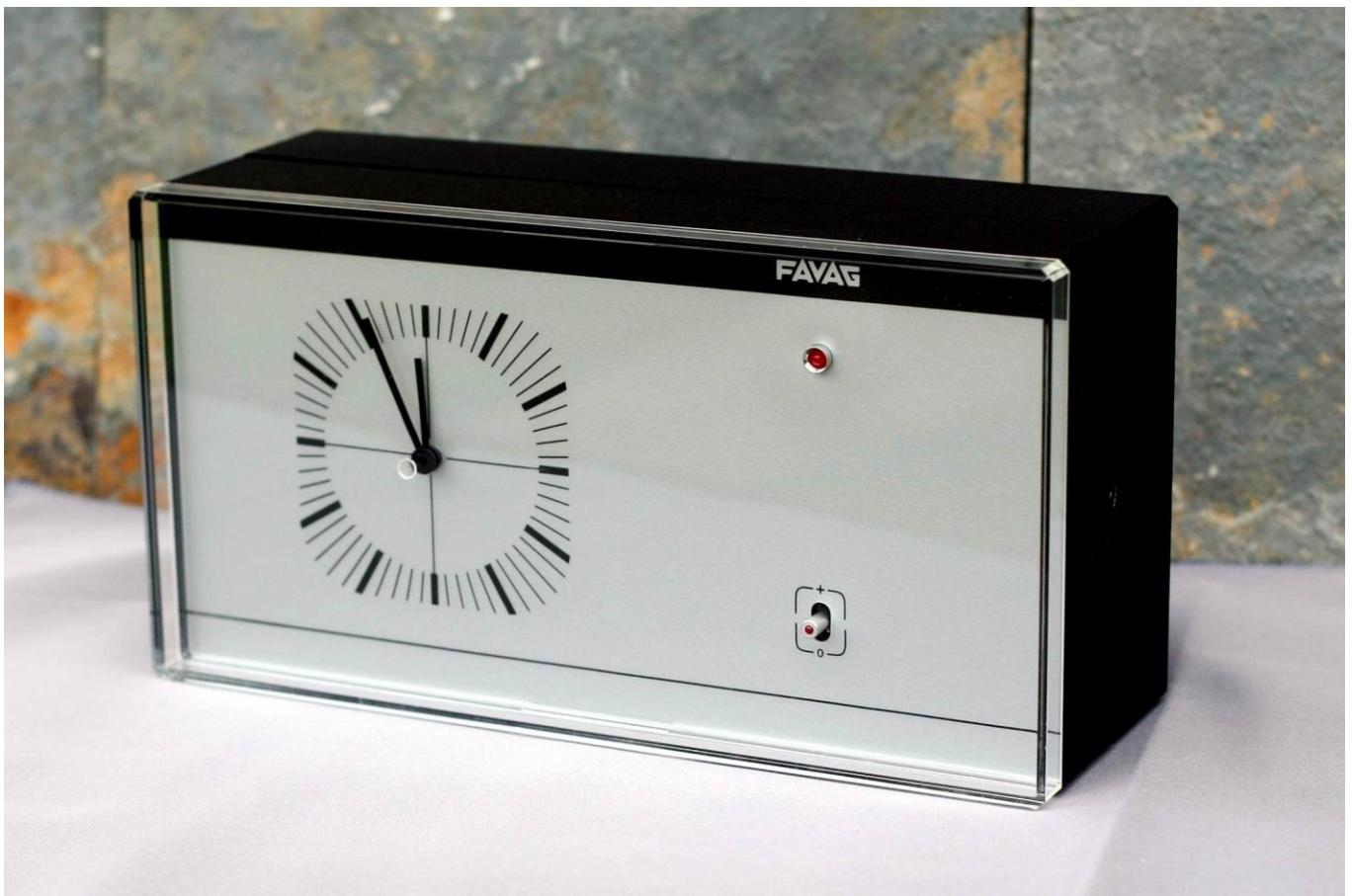
The Favag E 80 HBG is a radio controlled master clock with its own quartz timebase specified at 0.1 seconds in 24 hours at 20°C. The pilot dial in the image comprises a single stepping motor driving the motion work which can be run fast, stopped and started by means of a toggle switch.
