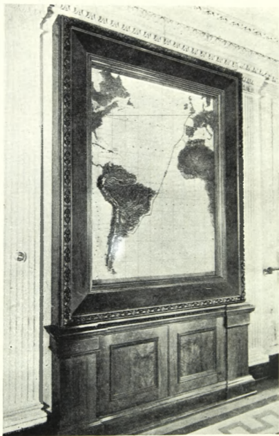
FIG. 131. "PUL-SYN-ETIC" AUTOMATIC SHIP'S POSITION INDICATOR
