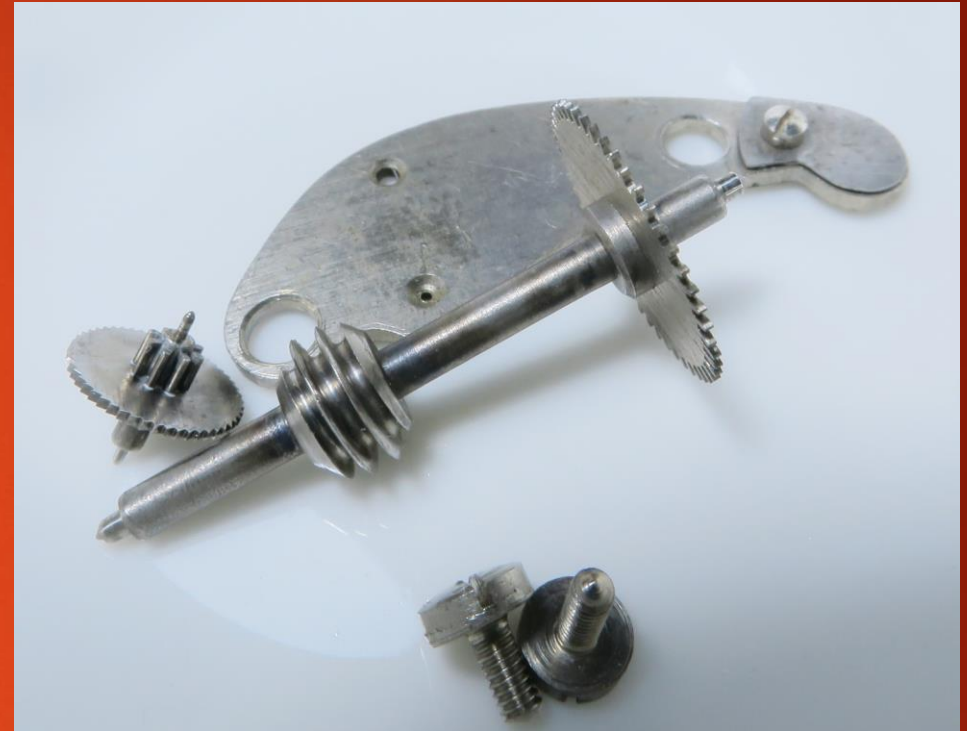
The escapement and electrical contact side 1
