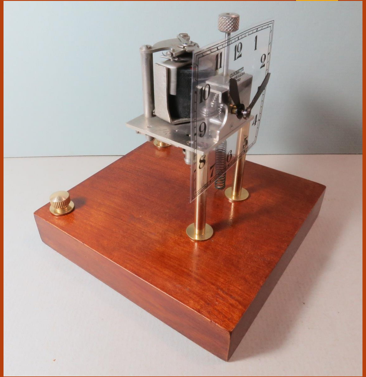
A simple base was constructed and a transparent dial added to display the movement
