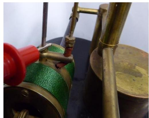
If the meter buzzes at each point then the circuit is good.
