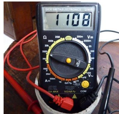
If the reading is “1” there is an open circuit in the coil and hence faulty.
