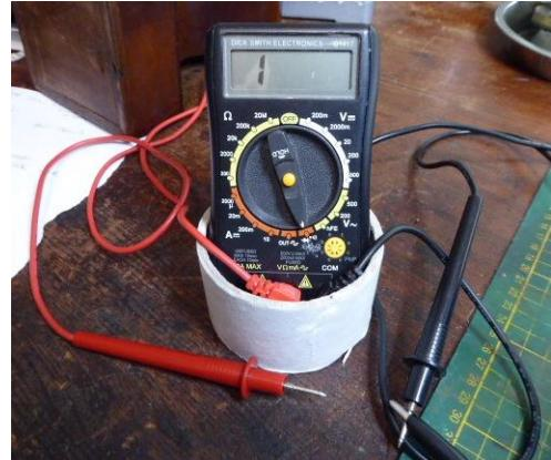
Using the red probe test each point of a connection on the clock frame and pendulum, following the negative side of the circuit right down to the entry to the coil.
