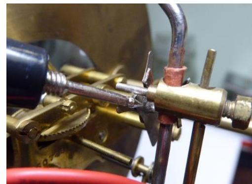
Release the pendulum to hang freely and place the probe on the silver contact pin holder.
