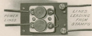
Cut showing block on top of the Master Clock to which the wires are attached
