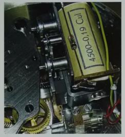
Fig. 29. Impulse coil and indexing mechanism.
