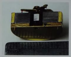
Fig. 24. Micro stepping motor with jewelled driving anchor.
