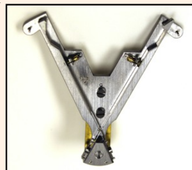
The special pallet arrangement of the Reid Escapement
