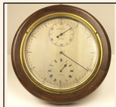
The regulator slave dial. There are two of these that are part of the clock..
