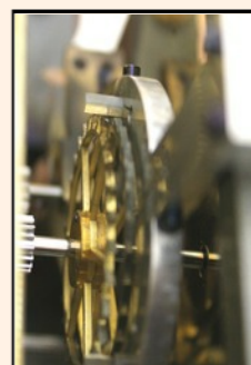
(right) A view of the double wheel escapement
