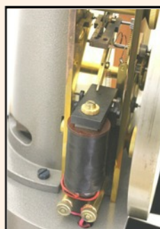
(left) The solenoid that sets the winding remontoire.
