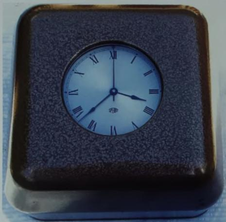
Fig. 13. Sperry prototype quartz chronometer for the Royal Navy.
